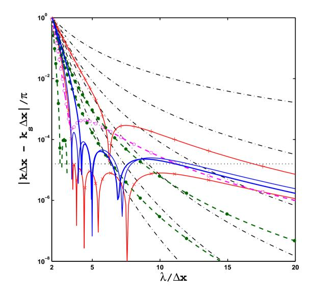
$ightarrow ext{error}$  observed for a harmonic wave  $e^{i(kx-\omega t)}$  propagating at  $v_{arphi} = \omega/k = ck_s/k$
