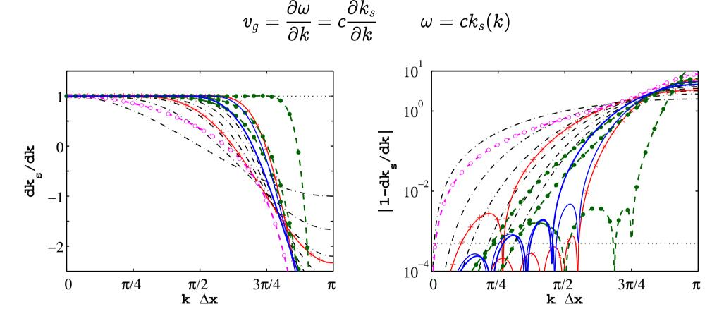
accuracy limit given by  $E_{v_q} = |\partial k_s / \partial k - 1| \le 5 imes 10^{-4}$
