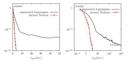
**Abstract** – A damped Newton algorithm for viscoelastic fluid flows is presented [1]. This algorithm bases on a projection formulation of the viscoplastic problem and an efficient preconditioned iterative solver for the singular Jacobian. A demonstration is provided by computing a viscoplastic flow in a pipe with a square cross section and performance are compared with the augmented Lagrangian algorithm.
