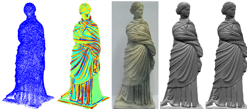
Figure 1: Initial raw point set; Point set curvature; Picture of the real object; Mesh obtained at coarse scale; Mesh back projected to a finer scale
