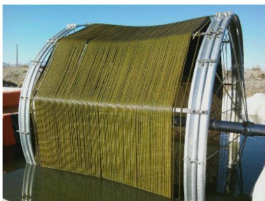
(a) Rotating microalgae biofilm device
