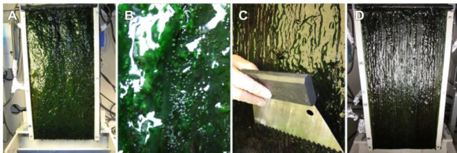
**Fig. 2** The vertical phototrophic biofilm reactor (**a**), a close-up of the biofilm before harvesting (**b**), harvesting part of the biofilm with the adhesive comb (**c**), and the biofilm setup after harvesting (**d**)
