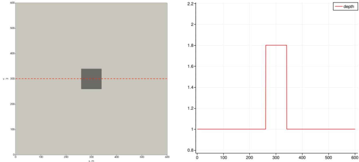
**Figure:** Initial condition of a 2D Riemann problem for the extended SGN model. Initial water depth is  $h_l = 1.8 \text{ m}$  inside the dark gray region  $\{(x, y) : 260 \text{ m} < x, y < 340 \text{ m}\}$  and  $h_r = 1.0 \text{ m}$  outside. Initial velocity is  $u_0 = v_0 = 0 \text{ m/s}$ .
