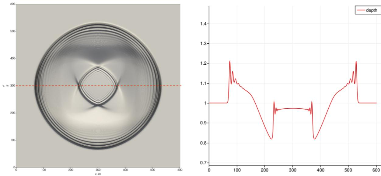
Figure: Numerical solution to 2D Riemann problem for the extended SGN model,  $t = 20\text{s}$ .
