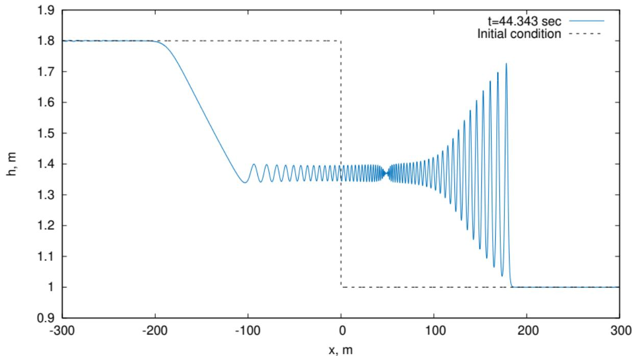
**Figure:** Numerical solution to 1D Riemann problem for the extended SGN model: a dispersive shock wave.  $N_{\text{cells}} = 8000$ ,  $\lambda = 300 \text{ m}^2/\text{s}^2$ ,  $t = 44.434 \text{ s}$ .
