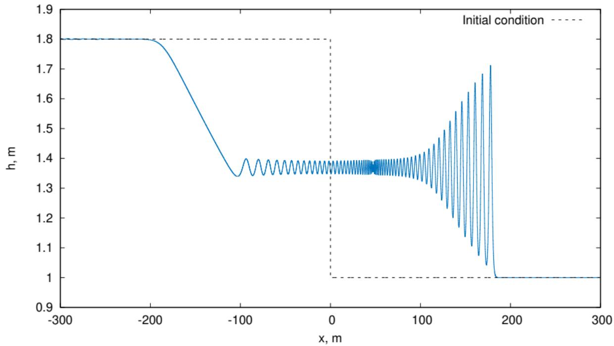
Figure: Numerical solution to the Riemann problem: Dispersive shock wave.  $N_{\text{cells}} = 768000$ ,  $\lambda = 300 \text{m}^2/\text{s}^2$ ,  $t = 44.434 \text{s}$ .
