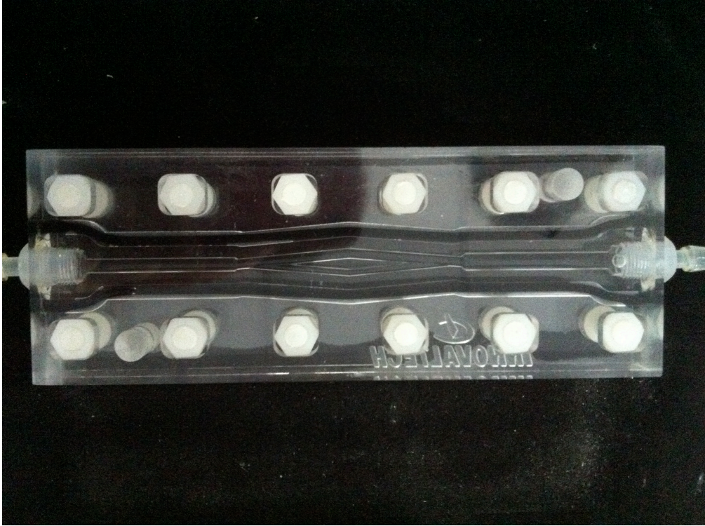
Figure 2: Physical phantom for cerebral arteries.
