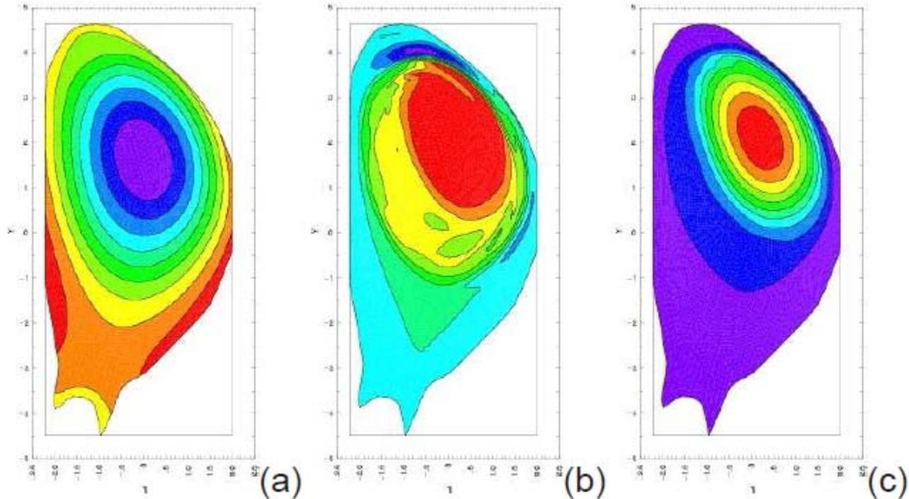
(a) Poloidal flux, (b) toroidal current, and (c) temperature during a vertical displacement event. A VDE brings the plasma to the upper wall where a  $(m,n) = (1,1)$  kink mode grows. Forces on the vacuum vessel are calculated.
