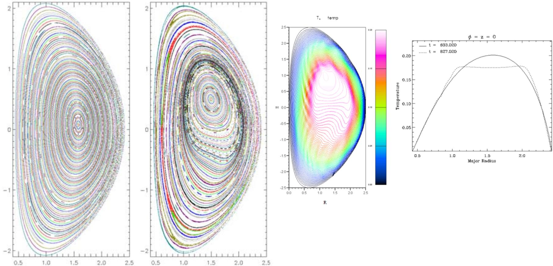
Saturated  $n=1$  mode can set develop when  $q_0$  slightly  $> 1$ , as seen in Poincaré plot on left. Can flatten temperature (right) and also drive  $m=2$  islands.
