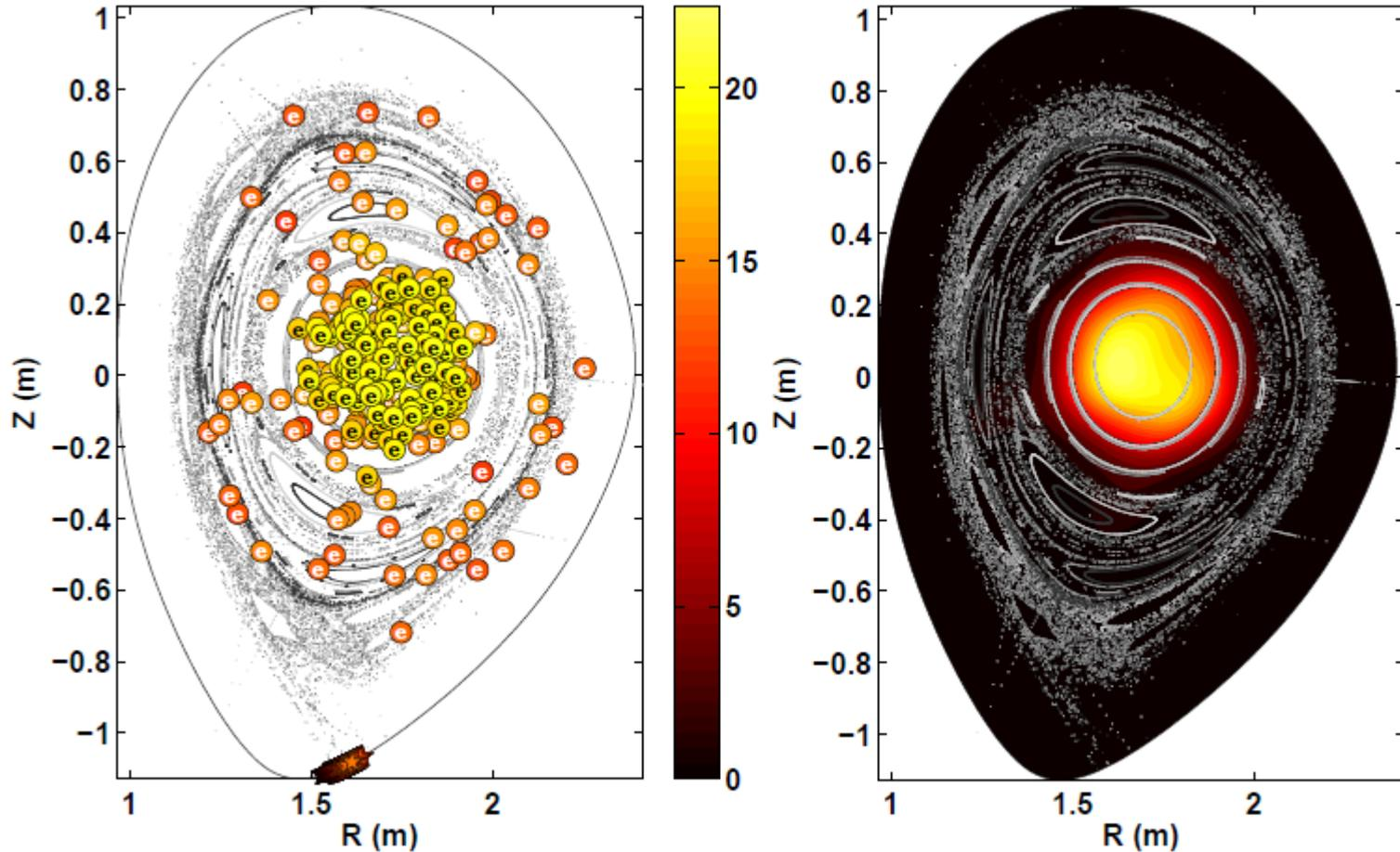
Simulation of DIII-D Ar pellet experiments. Runaway electrons of different energy shown. Synchrotron emission on right.
