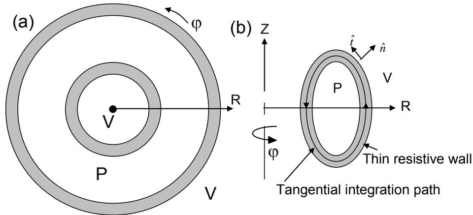
New instabilities can be present if the plasma is surrounded by a thin resistive wall. This can be modeled by modifying the boundary conditions.
