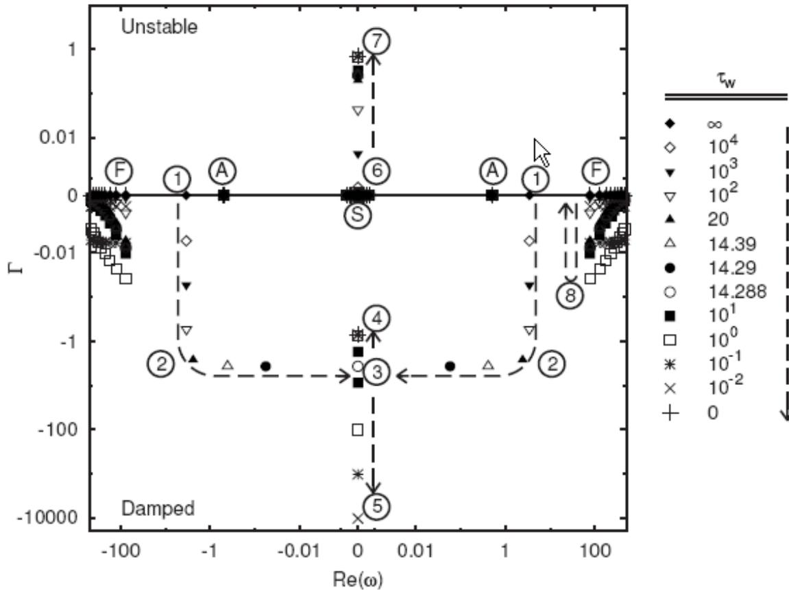
With sufficient plasma flow, the unstable mode will stabilize due to doppler shifted resonance with sound continua
